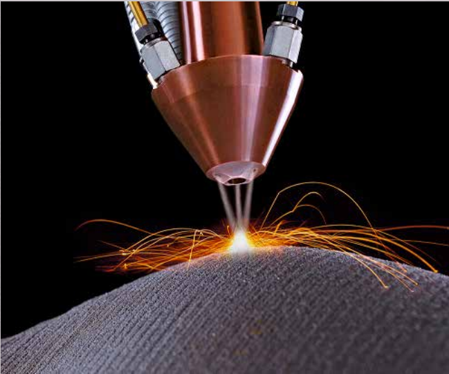
Figure 2: Laser cladding is an additive manufacturing process
