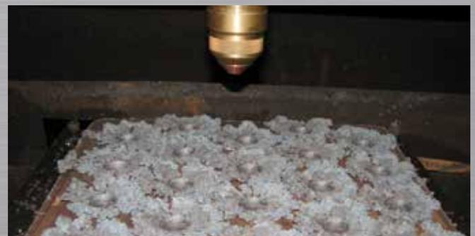
Figure 4. 1.75” 304L pierced with 400A H35 plasma. Slag piles resulting from piercing, note the pile height exceeds standard cut height for torch.
