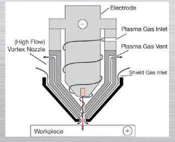
Figure 5. Hyflow<sup>™</sup> Vortex Nozzle
