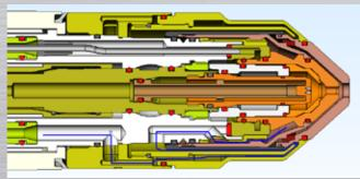
Figure 7. New: Liquid-cooled shield technology repels molten metal during piercing
