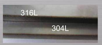
Figure 3. The results of using the 304L process settings for both 304L 5 mm and 316L 5 mm are demonstrated here
