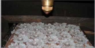
Figure 4. 1.75" 304L pierced with 400A H35 plasma. Slag piles resulting from piercing, note the pile height exceeds standard cut height for torch.
