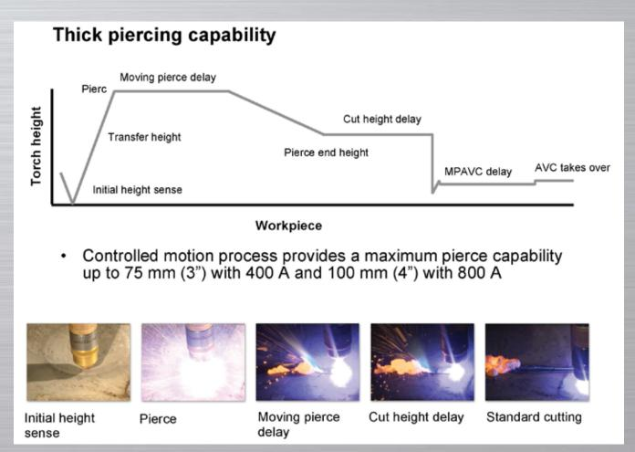
Figure 8. Thick Pierce Diagram
